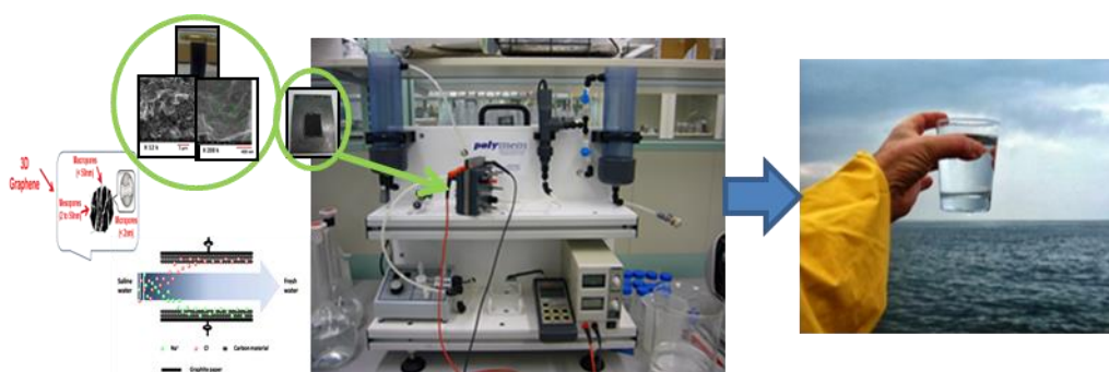
Fig. 1. Graphene based CDI pilot plant for desalination
